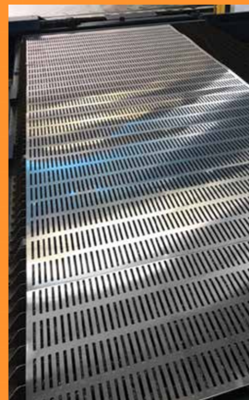
A skeleton from nose bridges produced on .025" 3003 aluminum.
