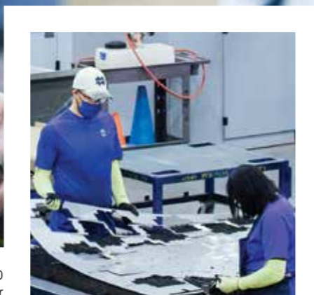
Employees work to identify parts cut on the TruLaser Tube 7000 and remove parts cut on the TruLaser 5030 fiber
