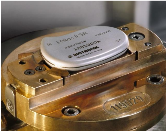
Figure 1: Heat-sensitive implants such as electronic pacemakers can be reliably sealed using laser welding. Pulsed lasers accurately produce a tight weld seam without overheating the pacemaker.
