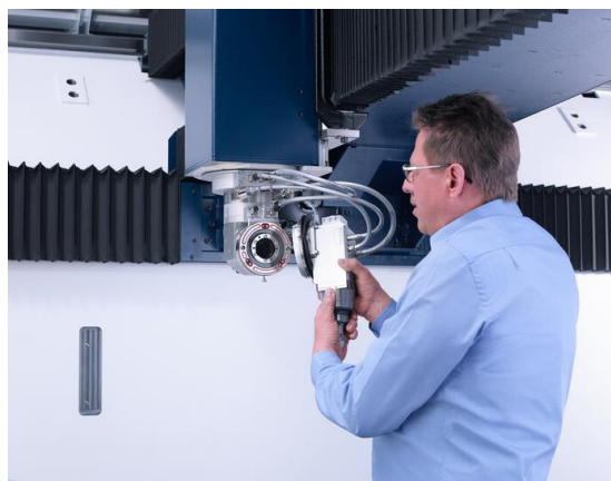
Figure 2: Magnetic clutch for collision protection and quick optics changeover.
