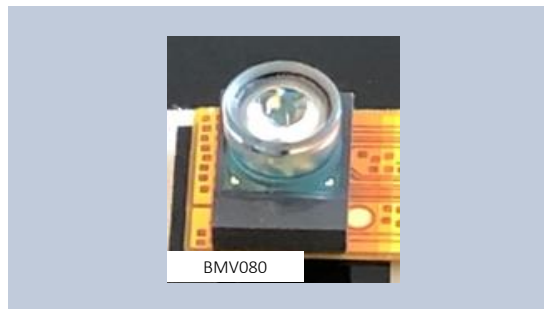
Figure 16: Miniature PM2.5 module with three VCSELs, optics and ASIC (BMV080 from Bosch Sensortec)
