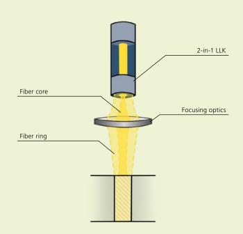
A laser with a greater than standard beam quality is used for BrightLine Speed\*. In addition, the laser is equipped with a wedge beam switch to generate special power distribution between the core and the ring in the patented 2-in-1 optical laser cable. Influencing factors which before had seemed conflicting are now combined thanks to the completely altered power distribution. This elevates the process to a new, application-specific level.
